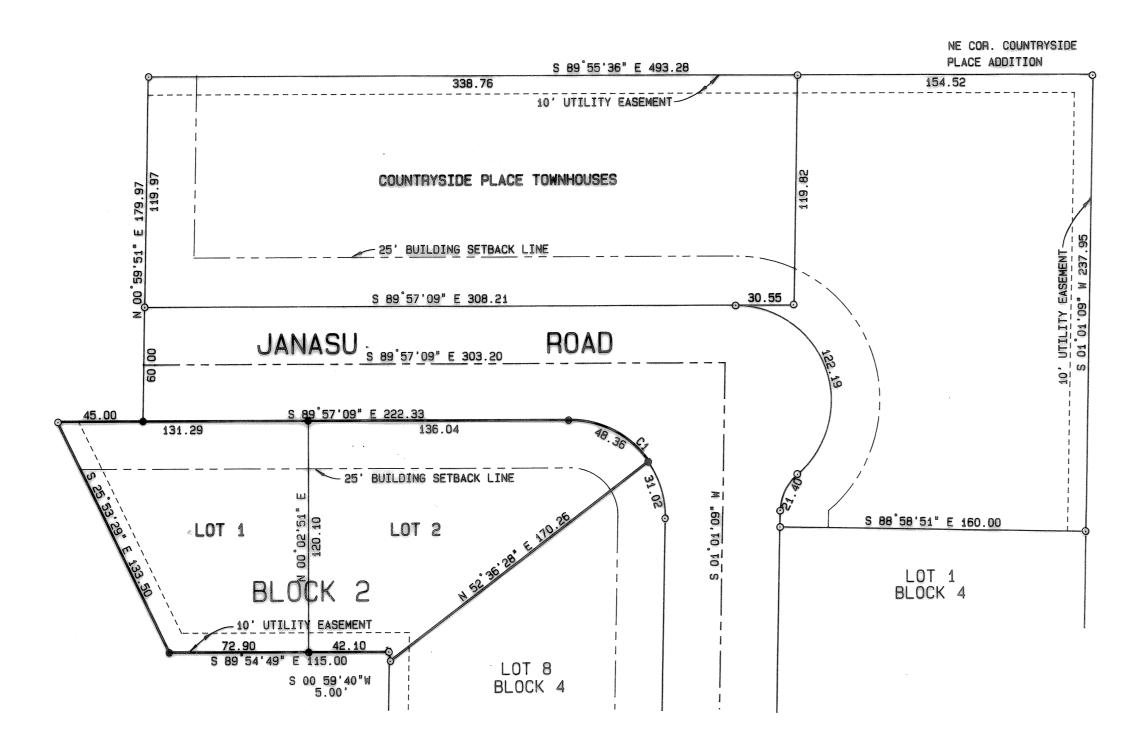
NOTE: SIDEWALKS SHALL BE INSTALLED IN BACK OF THE CURB ON THE SOUTH SIDE OF JANASU ROAD IN ACCORDANCE WITH CITY SPECIFICATIONS AND GRADE. INSTALLATION OF SIDEWALKS SHALL BE CONCURRENT WITH THE HOUSING CONSTRUCTION ON SAID BLOCK 2, COUNTRYSIDE PLACE.
